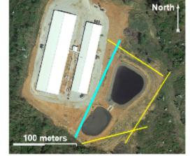
Holding Transect Ponds MTJ108 This transect has a 3.0 meter spacing between the electrodes (1.5 meter resolution).
