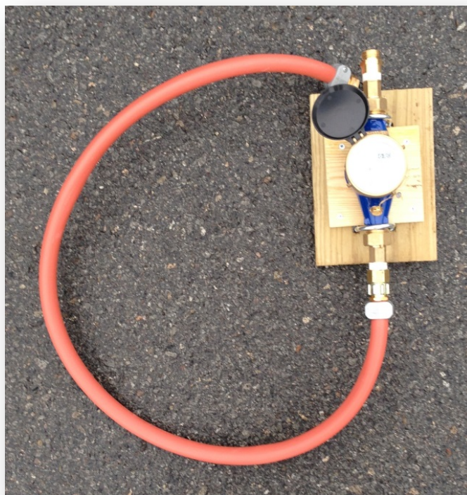
Figure 9. Standard water meter with hose adapters and mounting base installed to measure water use during pressure washing to clean animal pens.
