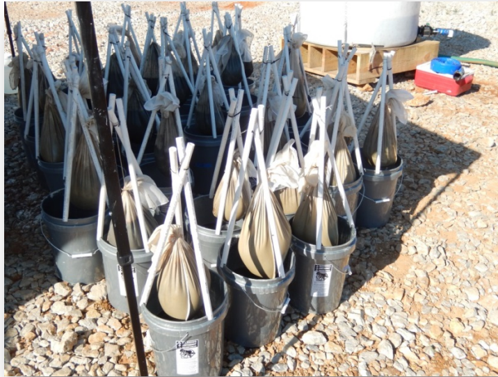
Figure 15. Filter bags containing separated manure slurry suspended above their respective buckets of leachate.
