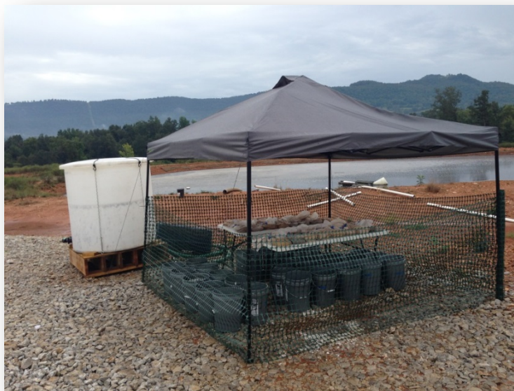
Figure 16. Leachate buckets and filter bags after the separated solids were dry enough for placement on tables for additional drying.
