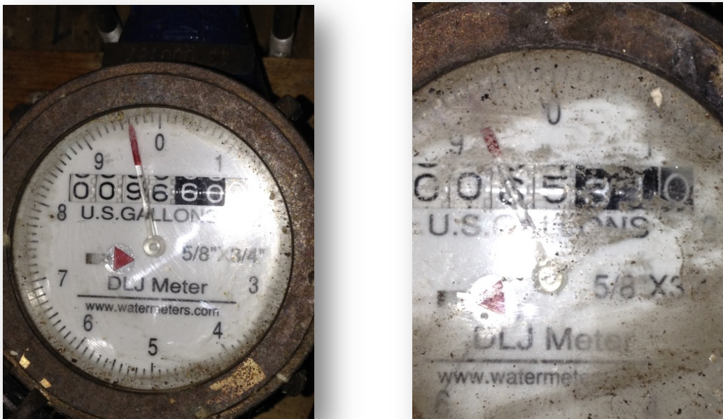
Figure 11. Two water meters purchased and installed on March 20 th , 2014 to measure pen wash down water additions to manure volume. Meters readings were 96,609.6 and 65,319.3 gallons for meter 1 and 2 on September 10 th , 2014.
