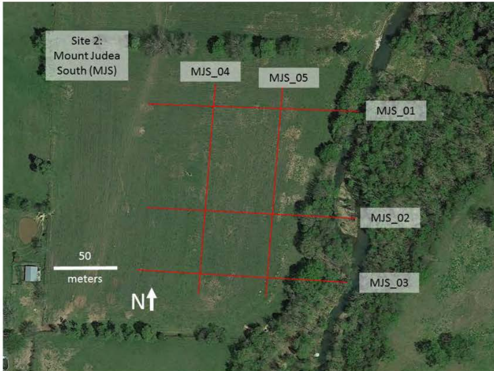
Figure 2. Location of ERI lines at southern (upgradient) site MJS. Five 165 meter long lines illustrated. 3 additional high resolution lines (placement not shown) will be acquired after evaluating initial data.
