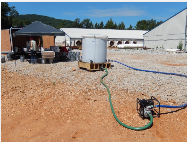
Figure 14. Manure collection and mixing system. Discharge valve for pulling manure for treatment is above the front corner of the tank base.
