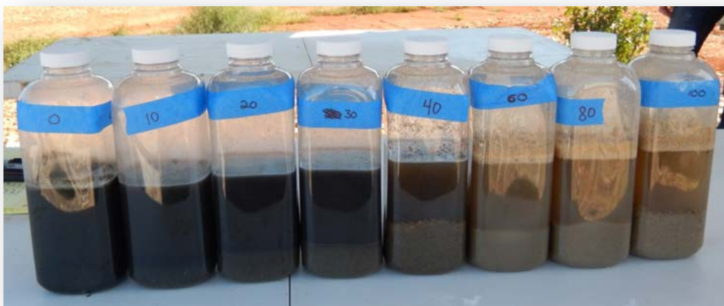
Figure 13. Calcium hydroxide slurry treatment test results. Bottle labels represent 0, 1, 2, 3, 4, 6, 8, and 10% Ca treatments. Based on both the clarity of the top liquid and settled solids a target rate of 5% was select for the chemical amendment trial.
