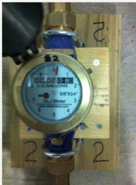
Figure 9. Two water meters purchased and installed on March 20th, 2014 to measure pen wash down water additions to manure volume. Initial meters readings were 126.6 and 80.2 gallons for meter 1 and 2.
