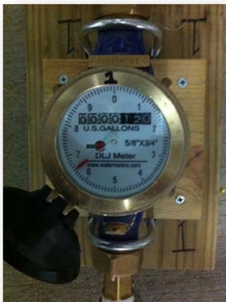
Figure 9. Two water meters purchased and installed on March 20th, 2014 to measure pen wash down water additions to manure volume. Initial meters readings were 126.6 and 80.2 gallons for meter 1 and 2.
