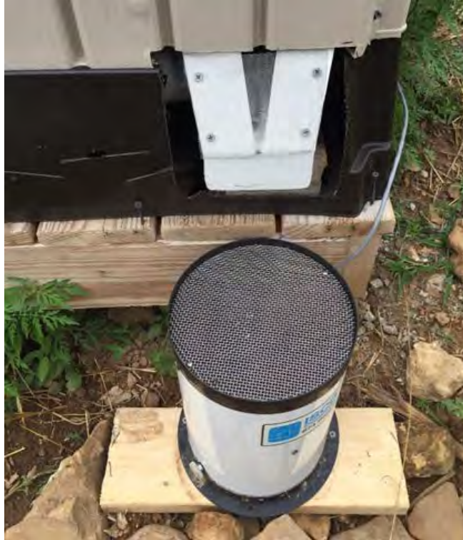
Figure 4. Tipping bucket rain gage to measure low interceptor trench flow (i.e., < \sim 12 mL/second).
