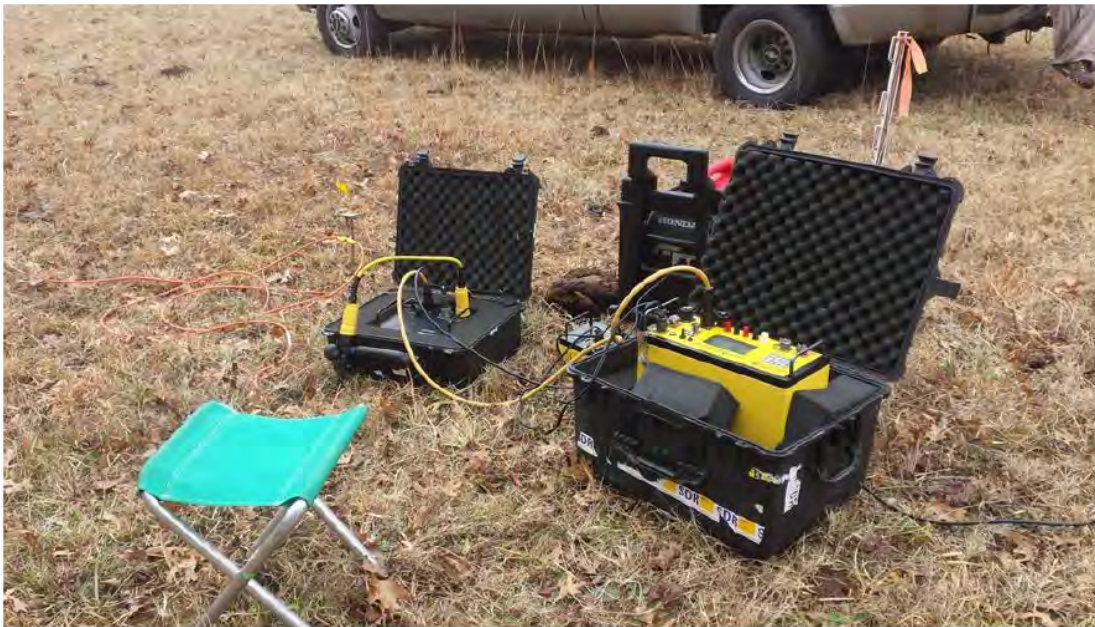
Figure 1 - Electrical resistivity equipment during data collection (12.17.14)
