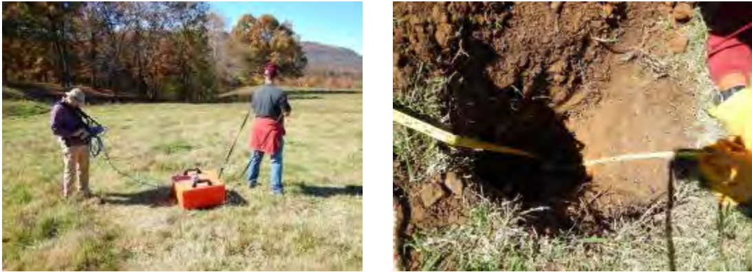
Figure 2. Conducting the Ground Penetrating Radar assessment at C&H Farm.
