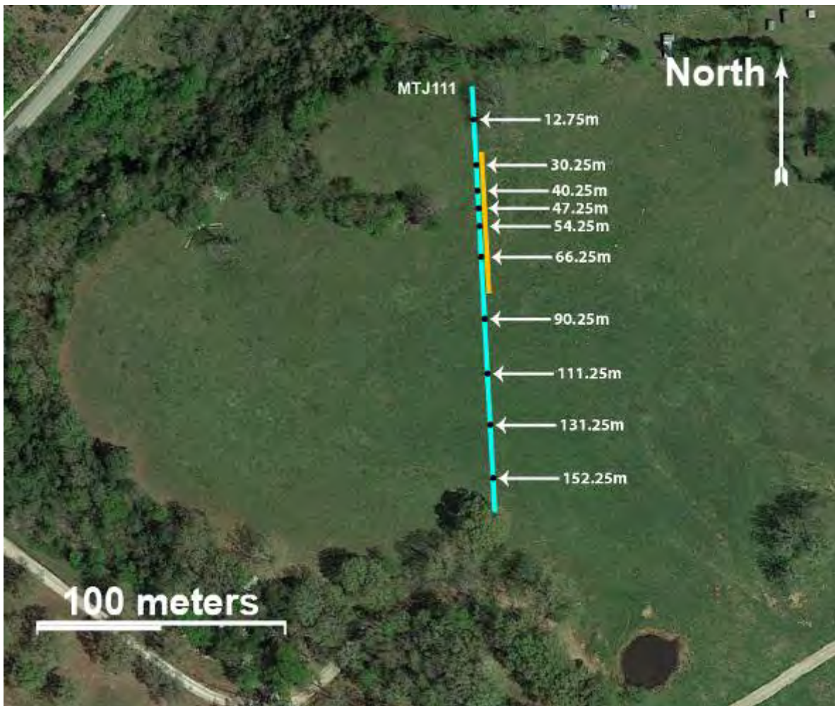
Figure 8 – Black dots represent soil sample locations along transect MTJ111 (blue line) on Field 1 (recent application site). Yellow line represent other ERI line collected at site.
