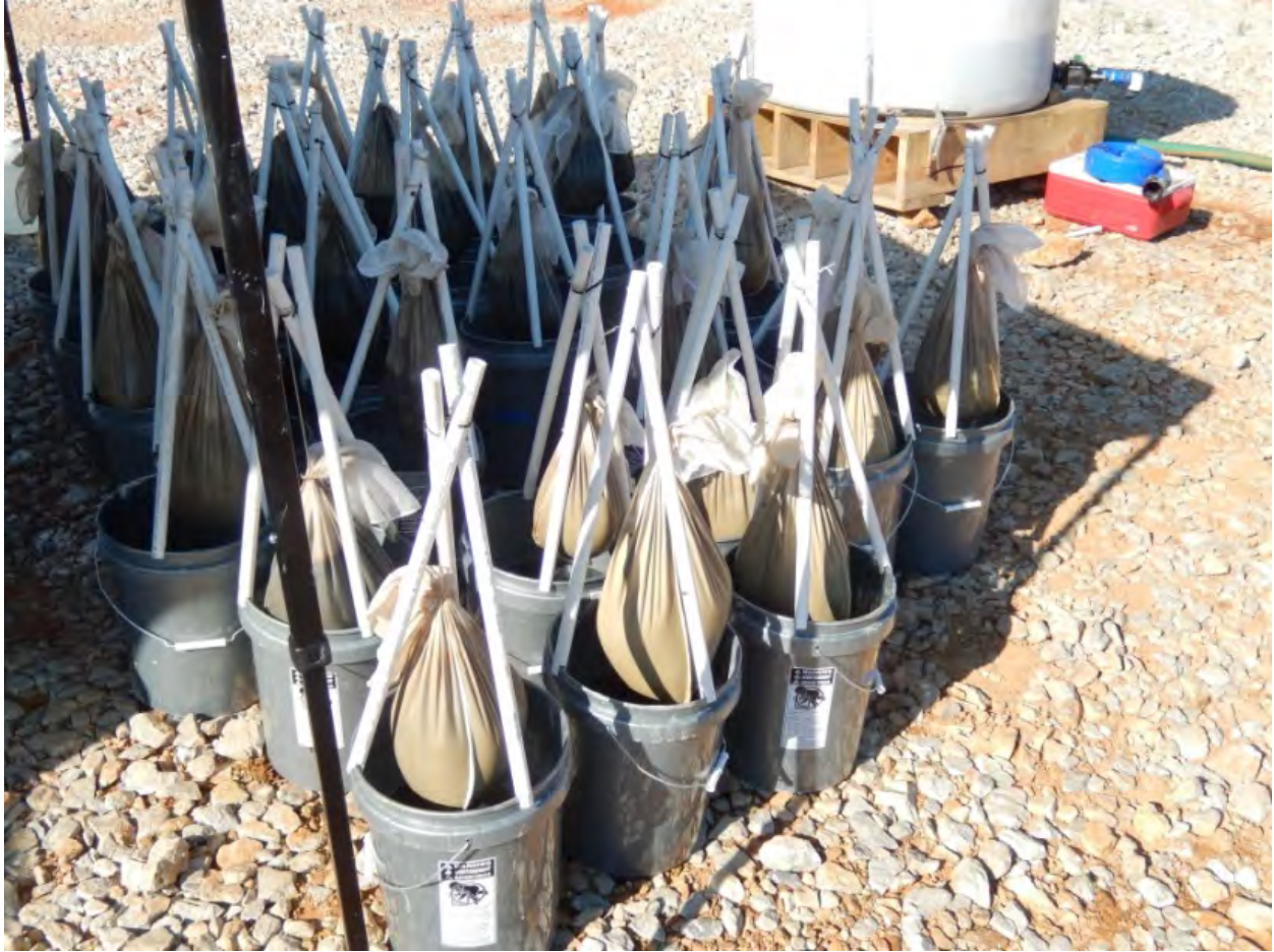
Figure S 4. Buckets containing manure leachate and suspended filter bags prior to being placed under awning for weather protection and 10-day storage.
