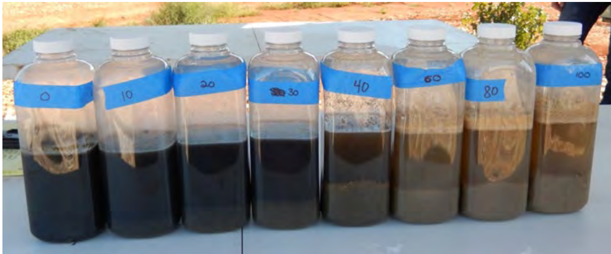
Figure 1. Clear test bottles after 30 % (wt/wt) Ca(OH) 2 slurry was added to 500 ml of manure at the rates of 0, 10, 20, 30, 40, 60, 80, and 100 mL/L and allowed to settle. Based on both the clarity of the top liquid and settled solids a target rate of 50 mg/L (5%) was select for the chemical amendment trial.
