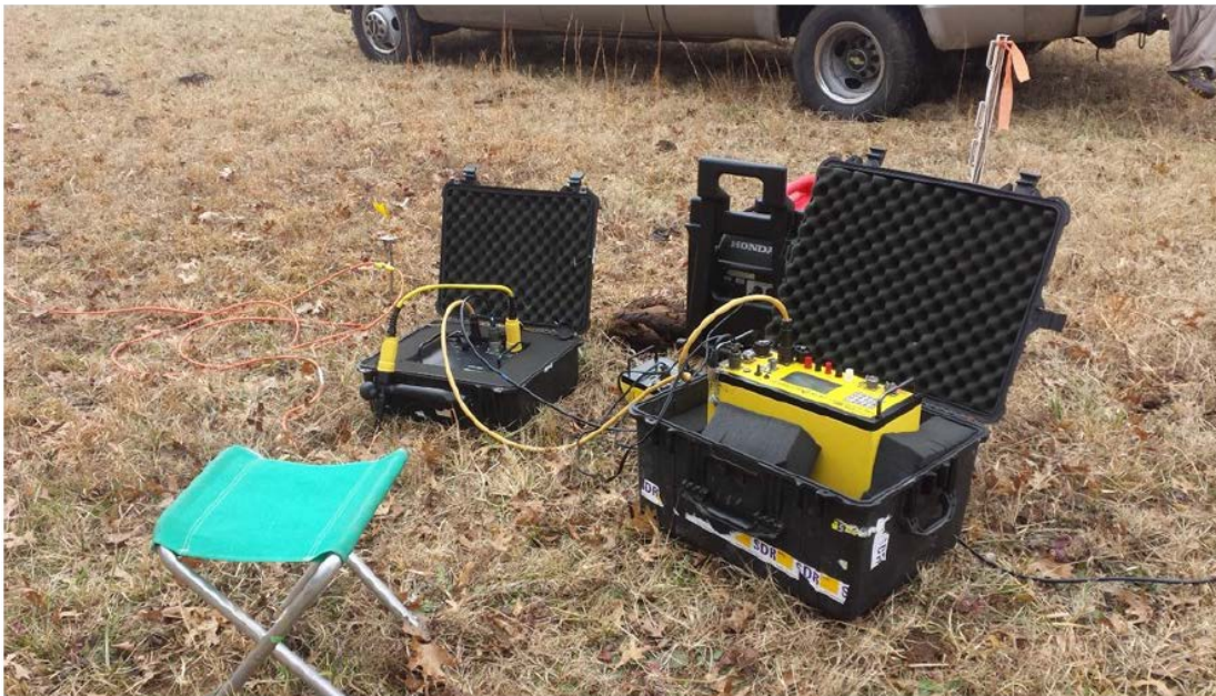
Figure 1 - Electrical resistivity equipment during data collection (12.17.14)
