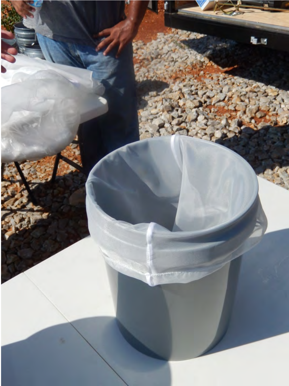
Figure S 3. Collection bucket lined with filter bag prior to addition of manure slurry and chemical amendment.
