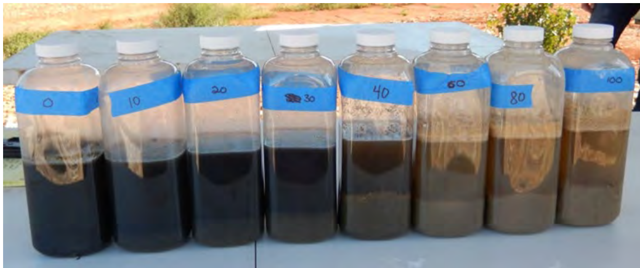
Figure 1. Clear test bottles after 30 % (wt/wt) Ca(OH) 2 slurry was added to 500 ml of manure at the rates of 0, 10, 20, 30, 40, 60, 80, and 100 mL/L and allowed to settle. Based on both the clarity of the top liquid and settled solids a target rate of 50 mg/L (5%) was select for the chemical amendment trial.
