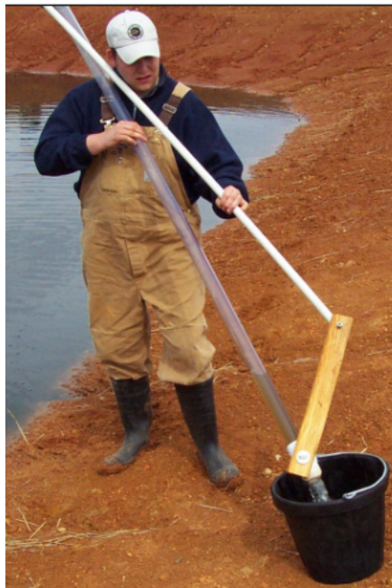
Figure 1. Foot valve manure sampler as used to collect samples from the C&H ponds.
